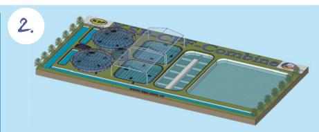
Farm planning with the water management system that proportionately divides the area into the water preparation pond, the culture pond, and the water treatment pond along with the adjustment in the farming method by separating the hatchery pond from the culture pond to facilitate pond cleaning.
